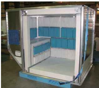
Refrigerated air-transport container developed using MechaCool
