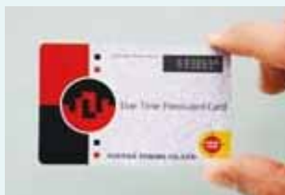
One-Time Password Cards use e-paper technology and are Japan's first identification IC cards to have a display window
